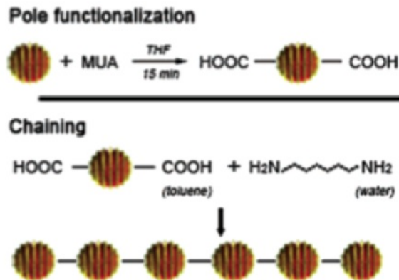
Figure 4.8 Functionalization and polymerization of striped nanoparticles into chains (33).
