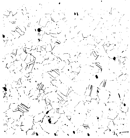
Fig. 56. Type 310 alloy, heat 25139. As received. 100x; cross section, etched electrolytically in chromic acid.
