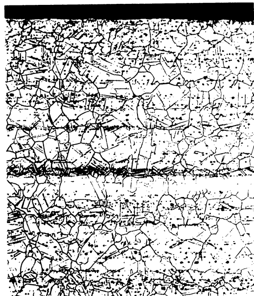
Fig. 64. Hastelloy B, heat B-1400. 1400°F, 100 hours, stress 10,000 psi. 75x; cross section, etched electrolytically in chromic acid.
