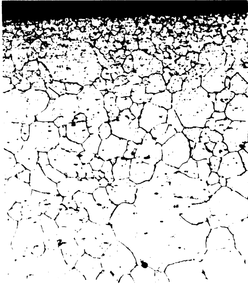
Fig. 55. Chromel alloy ASM, as received. 250x; cross section, etched electrolytically in 1-1-5 HCl, HNO 3 , H 2 O solution.
