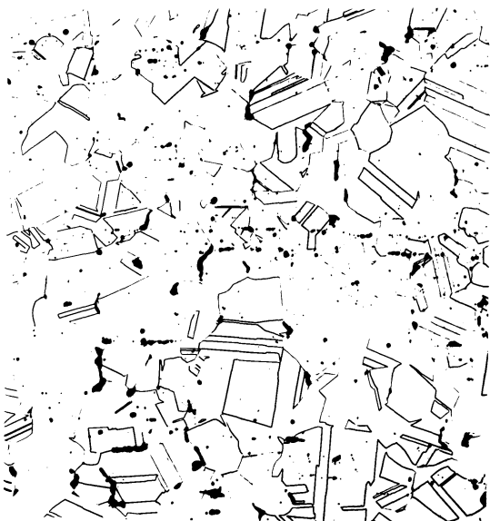
Fig. 61. Type 310 alloy, heat 25139. 1900°F, 100 hours, stress 755 psi. 100x; cross section, etched electrolytically in oxalic acid.
