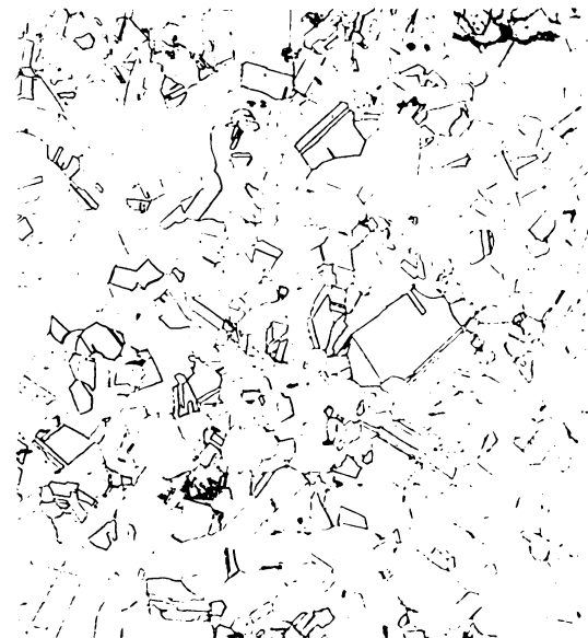
Fig. 58. Type 310 alloy, heat 4X-343. As received. 100x; cross section, etched electrolytically in chromic acid.
