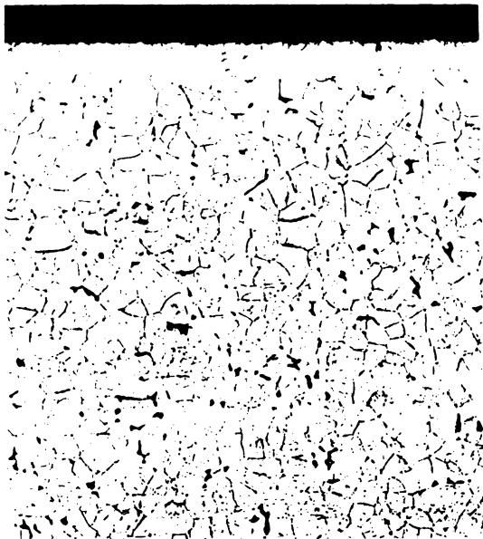
Fig. 59. Type 310 alloy, heat 25139. 1700°F, 100 hours, stress 2245 psi. 100x; cross section, etched electrolytically in oxalic acid.
