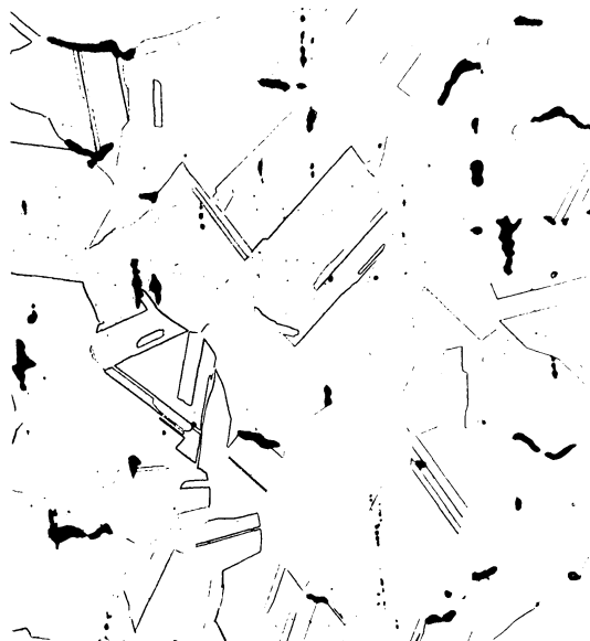
Fig. 62. Type 310 alloy, heat 25139. 2000°F, 100 hours, stress 755 psi. 100x; cross section, etched electrolytically in oxalic acid.
