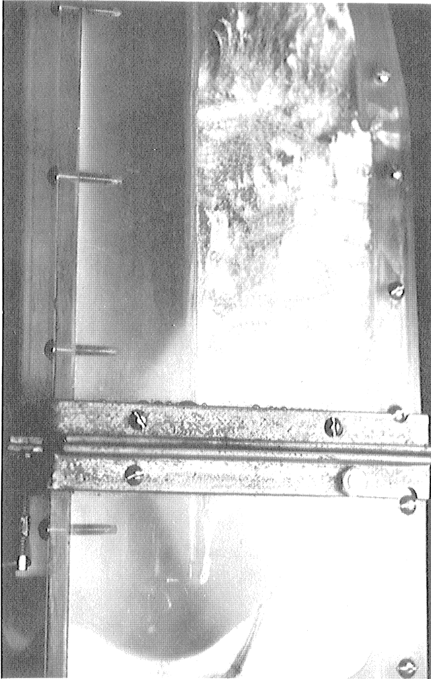
Figure 12. Air cleaner clogged with snow, no oil in cleaner.
