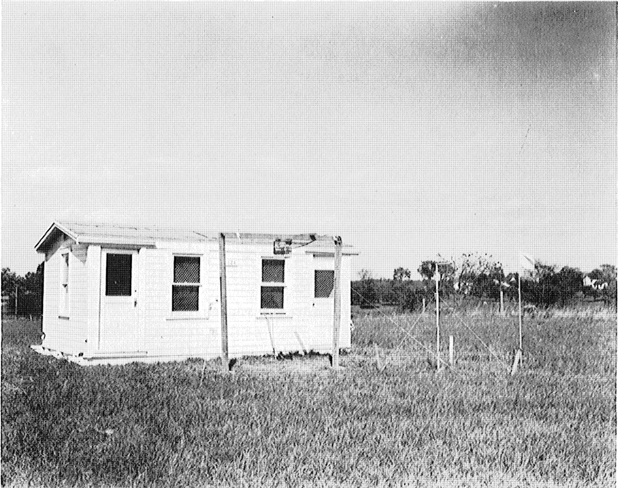
Figure 7. Field test house for ragweed pollen penetration studies showing outside instrumentation.
