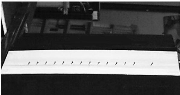
Fig. 7 Installed static VG test array; view from above and ahead of test article.
