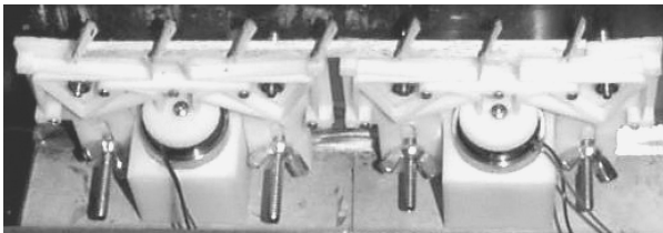
Fig. 8 High-frequency, deployable MVG test hardware.
