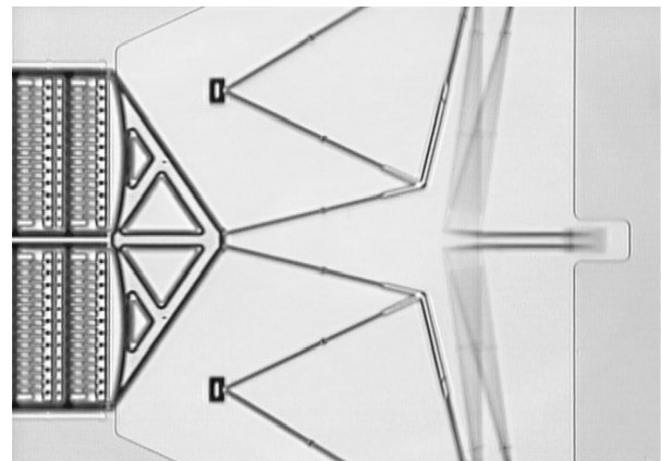
Fig. 5 Electrostatic actuator driving a compliant amplifier at 26.9 kHz.
