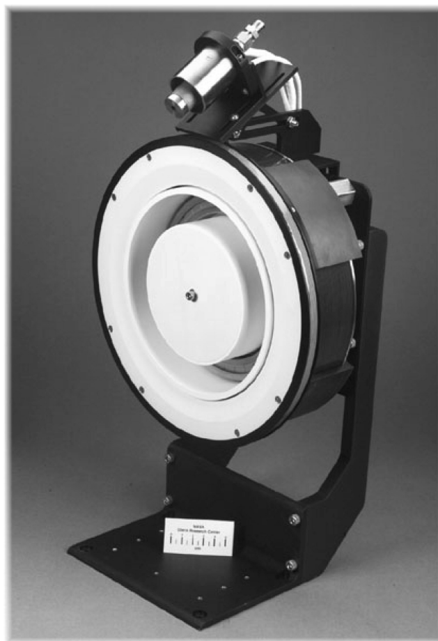
Fig. 1 High-specific impulse NASA-173Mv2 Hall thruster.
