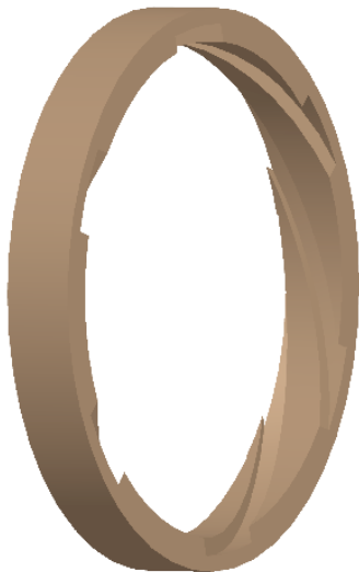
Figure 4. Schematic of ceramic rotor, showing inside-out helical ramjet channels.
