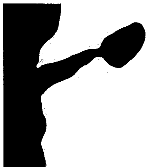
Fig.4 Typical shadowgraph of ligament tip (Rayleigh) breakup at the surface of round and annular free jets.
