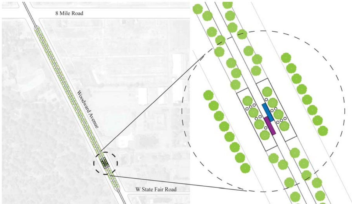
Figure 9.3: Plan view of a linear park along the light rail line on Woodward Avenue. The linear park provides ample width to accommodate the healthy growth of native trees within the public space of the city street (Lee 2010)
