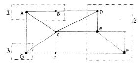
The system consisting of junctions A and B is enclosed by system boundary number 1. Similarly the system of junctions D E F is enclosed by boundary number 2. Junction G is in system boundary number 3.
