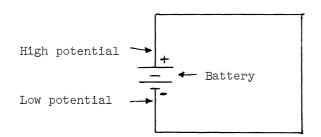
Electric current flows from points of high potential to points of low potential.
