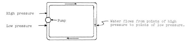
There is a very close analogy between this hydraulic system and an electrical system. In place of the water you may think of the electrons as flowing from one point to another. In place of the water pump you may think of an electrical pump called a <u>battery</u> or a <u>generator</u>. (We are all familiar with the batteries and generators in the motors of automobiles.)
