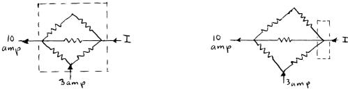
If the boundary is defined as shown above (right), it would cut other conductors, and I cannot be solved for directly. With the boundaries defined as shown in the figure on the left, you probably wrote the following equation:
