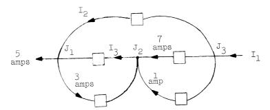
In this figure the boxes represent electrical appliances - heaters, lamps, etc. The value of the current is the same on both sides of the box.
