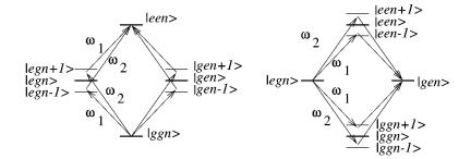
Figure 1.5: Graphical representation for a Sørensen-Mølmer gate. A bichromatic filed is applied with two frequencies summed up to  $2\omega_{eg}$ . Because both frequencies are detuned off the energy levels, the transitions occur only when two photons are absorbed or emitted. Different paths interfere with each other and eliminate the dependence of phonon population. (Figure from [55].)
