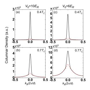
Figure 4.8: Momentum space columnar density along the x-axis in the first Brillouin zone, where clear bimodal structures appear for temperatures below  $T_c$ . Here, the solid curves are the total momentum density profile, and the dashed curves are the momentum density profile of the normal component. The trapping frequency used in these plots is  $\omega = 2\pi \times 60$  Hz, and the number density per site is unity at the trap center.
