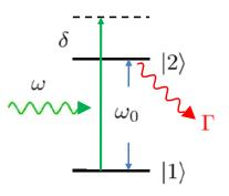
Figure 1.3: Two-level configuration for a neutral atom interacting with the laser field. In this illustration the spontaneous emission is neglected.
