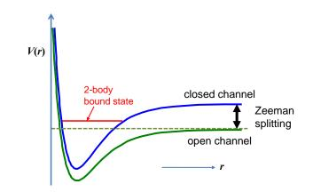
Figure 1.2: Energy diagram for a Feshbach resonance. The closed channel potential with a bound state is coupled to the scattered state continuum of the open channel. The degree of resonance can be adjusted by a magnetic field through Zeeman effects.
