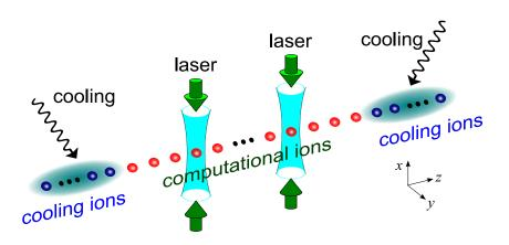
Figure 5.1: Linear architecture for large scale quantum computation, where lasers address individual ions and couple to local modes of the ions, while the edge ions are continuously Doppler laser-cooled. In a large ion chain, more efficient sympathetic cooling could be achieved with cooling ions sparsely distributed in the ion chain.
