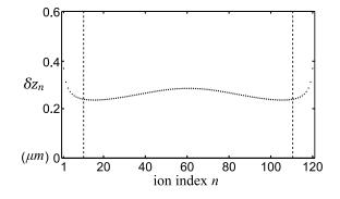
Figure B.1: The axial position fluctuation  $\delta z_n$  is plotted along the ion chain, which is about  $0.26\mu$ m (averaged) for the computational ions (*n* from 11 to 110).
