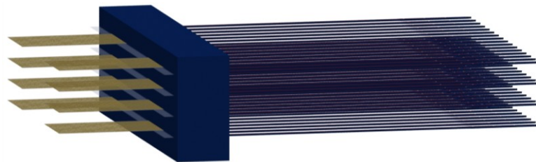
Fig. B.13: Conceptual drawing of the 256-site universal 3-D array.
