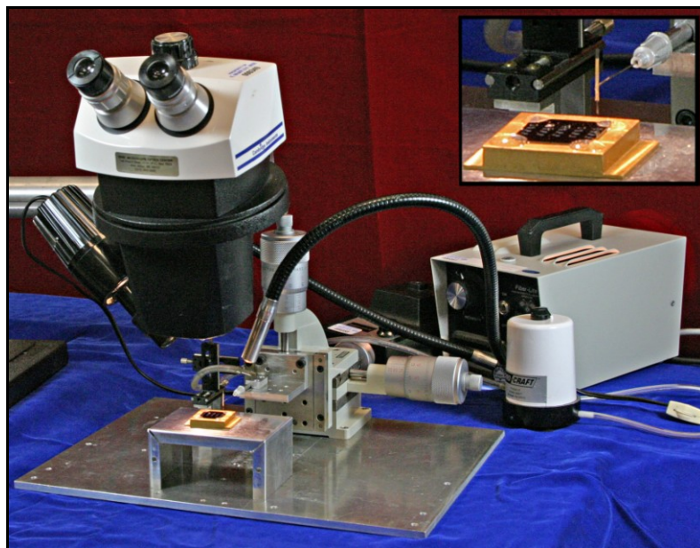
Fig. 6.16: Photograph of the assembly station. The inset shows a close-up of a probe on the vacuum wand and the assembly jig.
