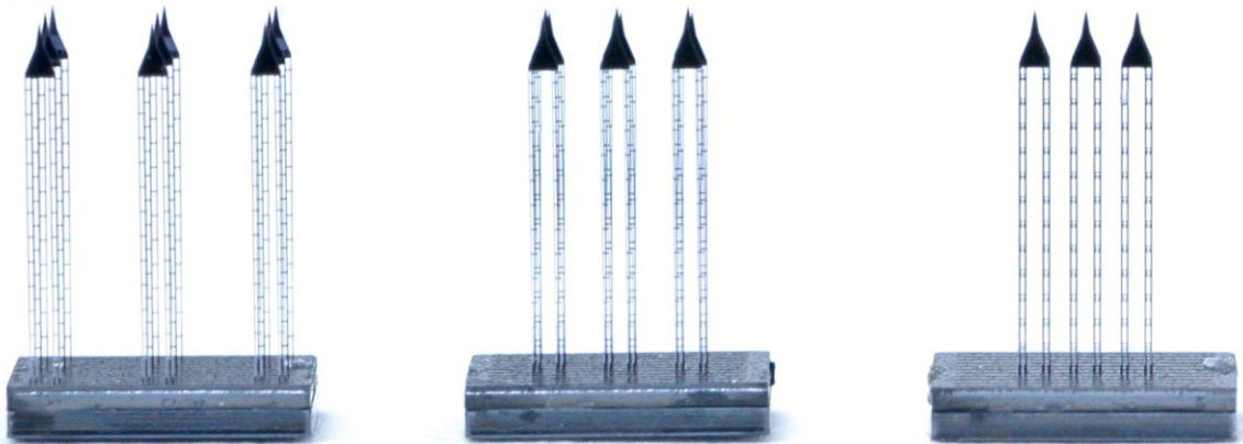
Fig. 2.32: Photograph of 300 \mu\text{m} -wide picket-shank 3-probe arrays with shanks and probes both spaced at 800 \mu\text{m} , 400 \mu\text{m} , and 200 \mu\text{m} (left to right).
