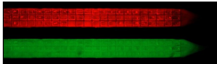
Fig. 2.21: Fluorescent images of coated lattice probes with tethered HPMA polymer functionalized with TexasRed labeled TT (top) and after further functionalization with FITC labeled NH 2 (bottom) [84].
