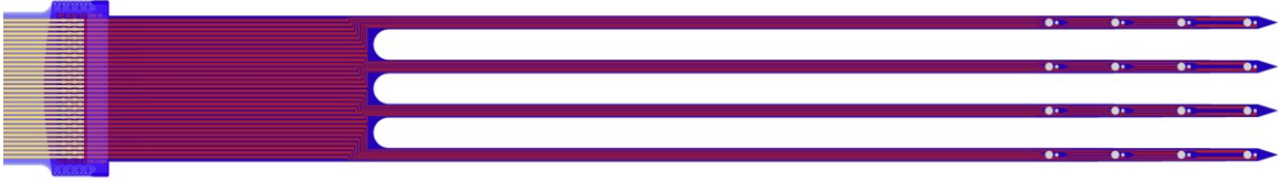
Fig. 6.3: Layout of a 32-site, four shank probe for recording and stimulation in VCN. The transition to the integrated cable at the probe back-end is also shown.
