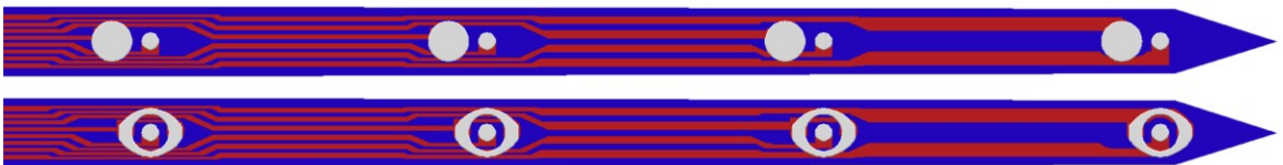
Fig. 6.4: Drawings of two VCN probe site configurations with adjacent (top) and concentric (bottom) arrangement for recording and stimulation.
