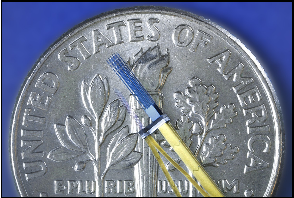
Fig. 6.23: Photograph of assembled 160-Site VCN-DCN 3-D electrode array on the back of a U.S. dime.
