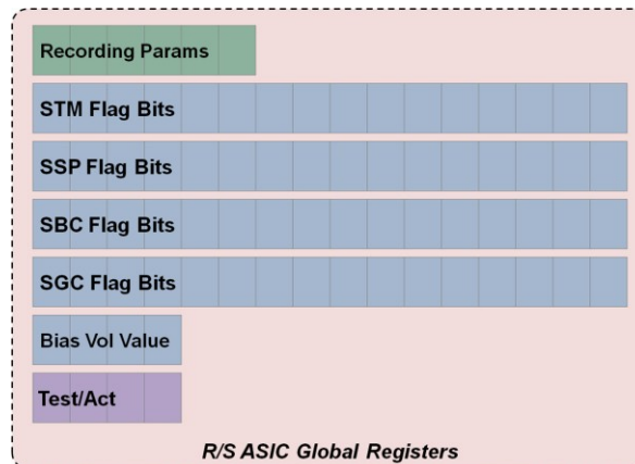
Fig. B.5: The global registers of the R/S ASIC.
