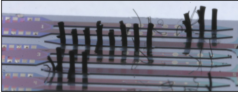
Fig. 3.16: Photograph of CNT growth (10min) on non-released probes. The taller forests clearly demonstrate the growth potential and have other applications including in work with in vitro cell cultures.
