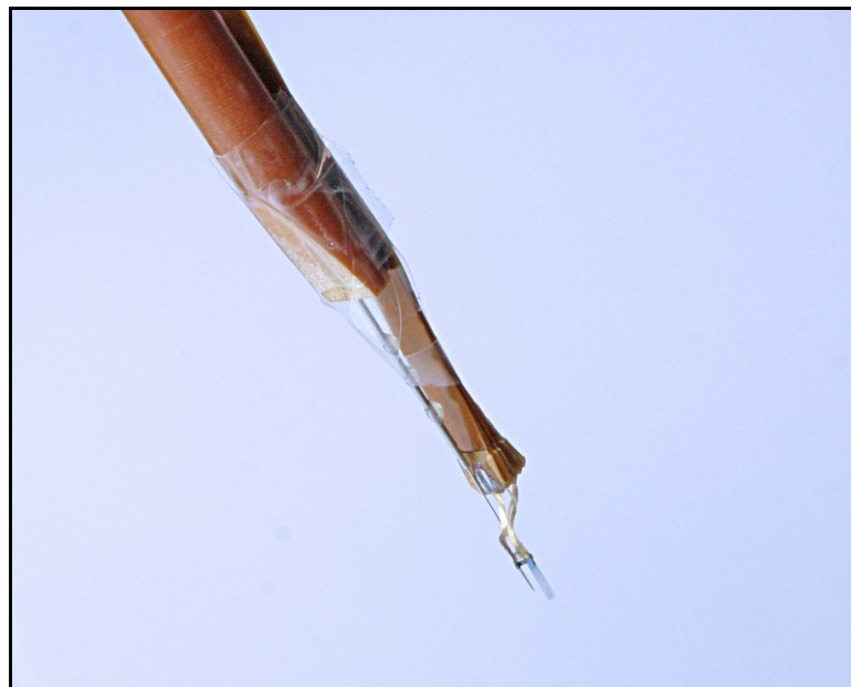
Fig. 6.22: Photograph of a 5-probe array after attaching to the insertion tool.
