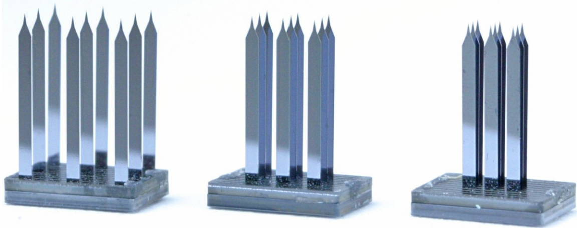
Fig. 2.31: Photo of arrays with 800 \mu\text{m} , 400 \mu\text{m} , and 200 \mu\text{m} spacings (left to right).
