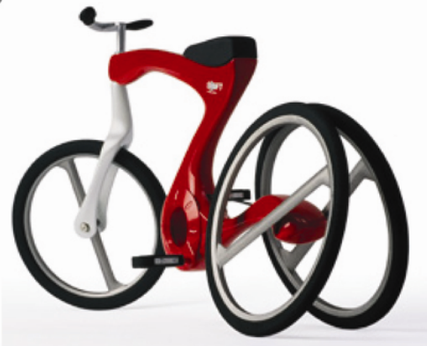
The wheels are shifted inwards to provide more balance to the bicycle at lower speeds and support stability.
