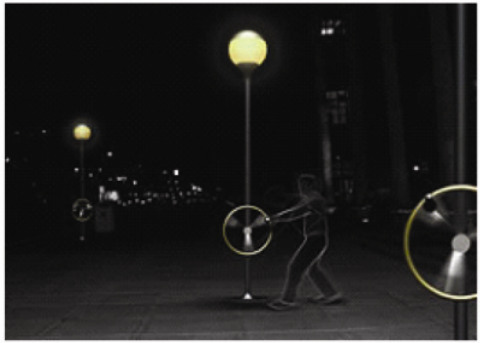
The sustainable street lighting system is composed of a network of street lamps collecting energy from pedestrians who take a turn at the crank-wheel to generate light.
