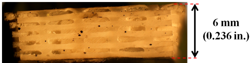
Figure 6.3 Through the thickness compression specimen, post failure image of the side view.
