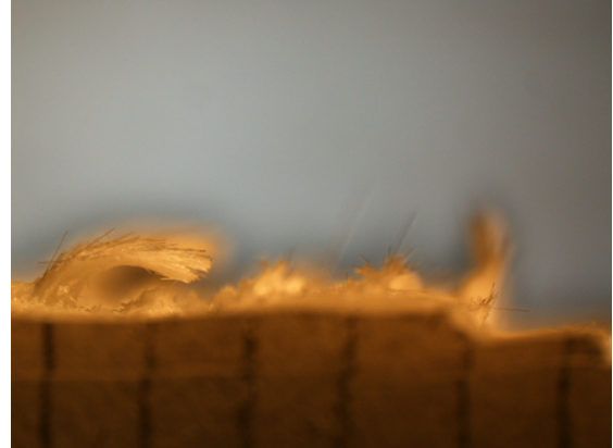
(a) Possible Z-fiber placement in ENF specimen. Notice the distinct points of Z-fiber (red color) and matrix (gray color) crossing the crack path.
