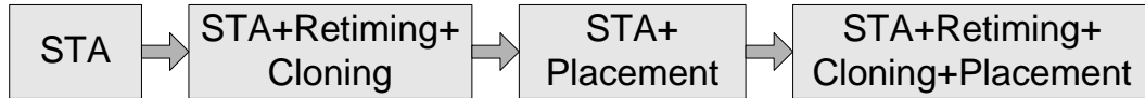
Figure 7.12: Our SPIRE flow proceeds in phases. First the MILP that represents only static timing analysis is solved without design changes. The values of relevant variables are saved and passed to the next stage which runs an MILP that incorporates retiming and cloning. The retiming variables are saved and fixed in an MILP that allows latches to move. Finally, with known values for latch locations and retiming variables we run the complete linear program.
