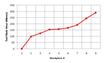
Figure 2.19 Tool flank wear of nine sample workpieces in experiment 1.
