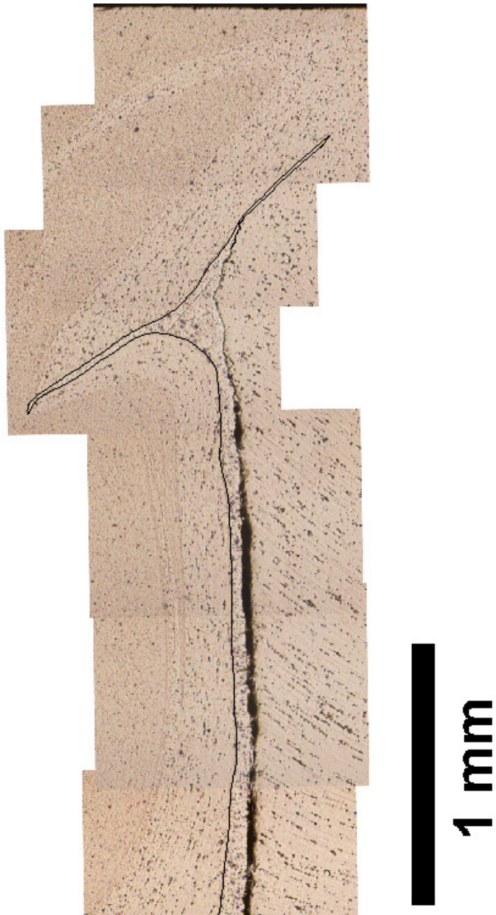
Fig. 2.3 A magnified portion of the foil in Fig. 2.2 where it is bifurcated due to complex flow within the weld zone.
