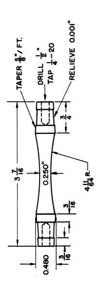
FIG. I FATIGUE TEST SPECIMEN
