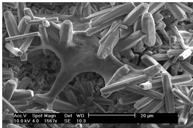
FIGURE 5. Scanning Electron Micrograph of DPSC cells grown on FA surface. At greater magnification shows cytoplasmic extensions of the cells adhering to the individual FA crystals.
