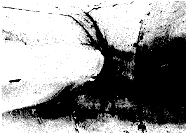
Figure I-5. A typical "mild" icing condition on the wing root of a B-24-type bomber. (175 mph, 6000 ft, -3^{\circ}\text{C} , drop diameter = 17 microns (avg), 0.2 grams of liquid water per cubic meter of air.
