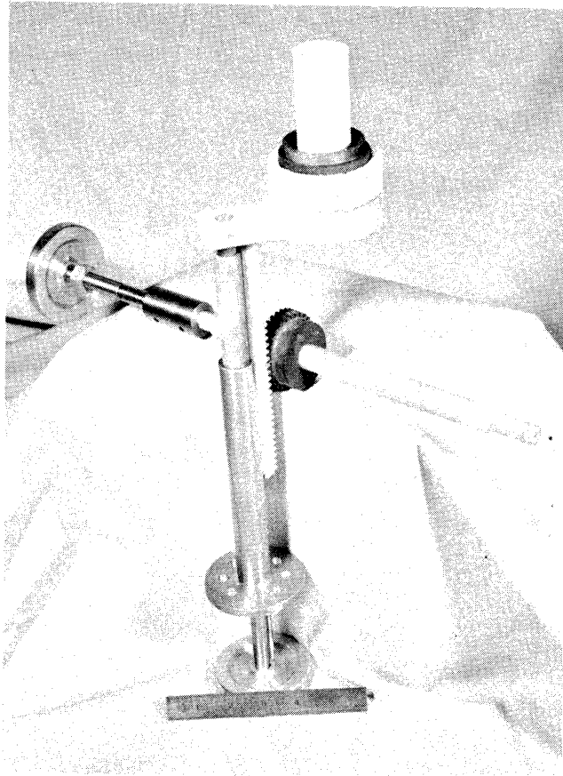
Figure 8. Lowering and Turning Mechanism Removed from the Pressure Vessel.
