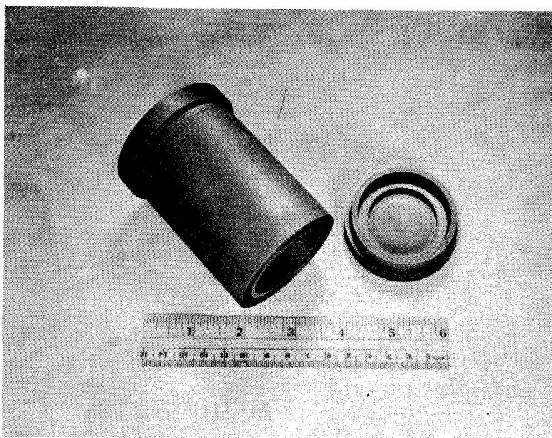
Figure 5. Graphite Susceptor Which Forms A Heating Chamber of Uniform Temperature.
