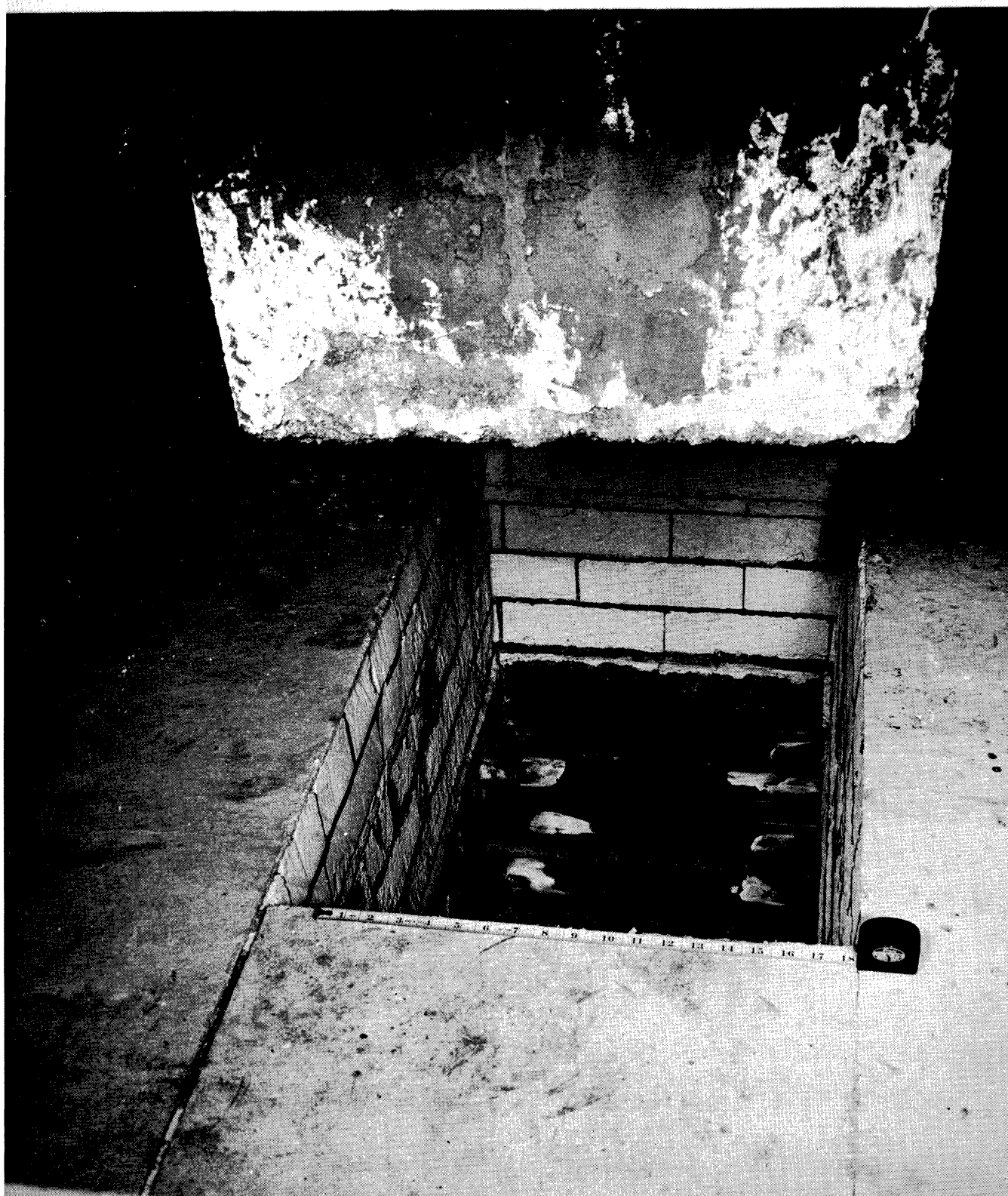
FIGURE I LOOP FURNACE ENCLOSURE AND HEATING ELEMENTS
