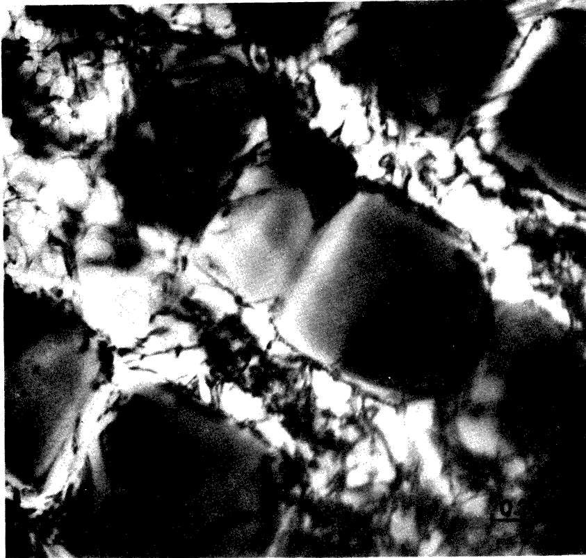
Figure 27. Thin foil electron micrograph of a smooth specimen of Udimet 700 bar solution treated, aged 4 hours at 1975°F (1079°C) plus 24 hours at 1550°F (843°C) plus 16 hours at 1400°F (760°C) and creep-rupture tested at 1200°F (649°C) at 110 ksi (758 MN/m 2 ).
