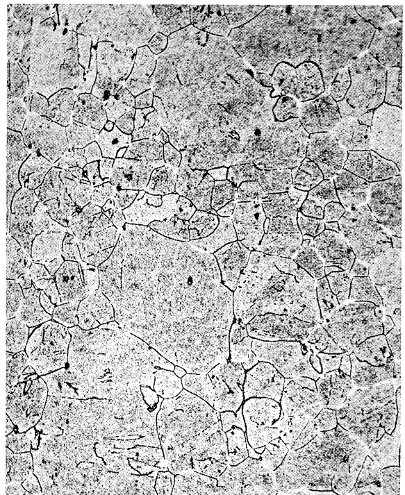
Figure 42. 100X Aged 10 hours at 1700°F
