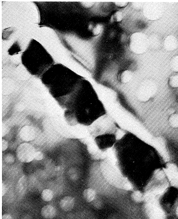
Figure 51. Electron micrographs showing \gamma' and carbide precipitates in the grain boundary of 0.026-inch thick Waspaloy sheet solution treated 1/2-hour at 2150°F and aged 10 hours at 1700°F.
