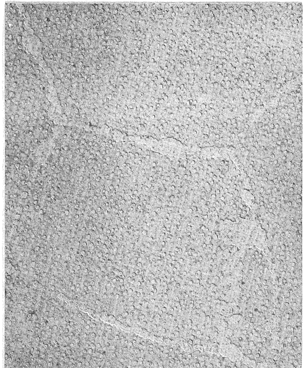
Figure 46. 5,400X Aged 10 hours at 1700°F Solution Treated 1/2-hour at 1900°F
