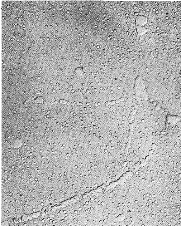
Figure 43. 5,400X Aged 16 hours at 1400°F Solution Treated 1/2-hour at 1825°F
