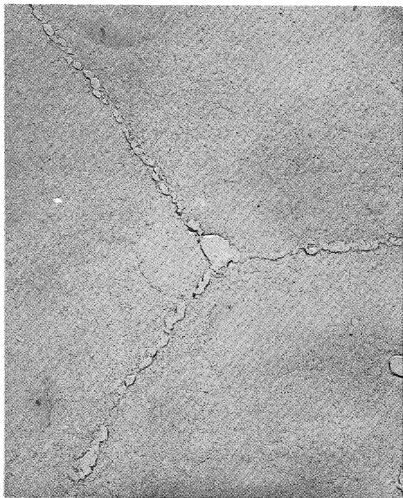
Figure 47. 5,400X Aged 16 hours at 1400°F Solution Treated 1/2-hour at 1975°F
