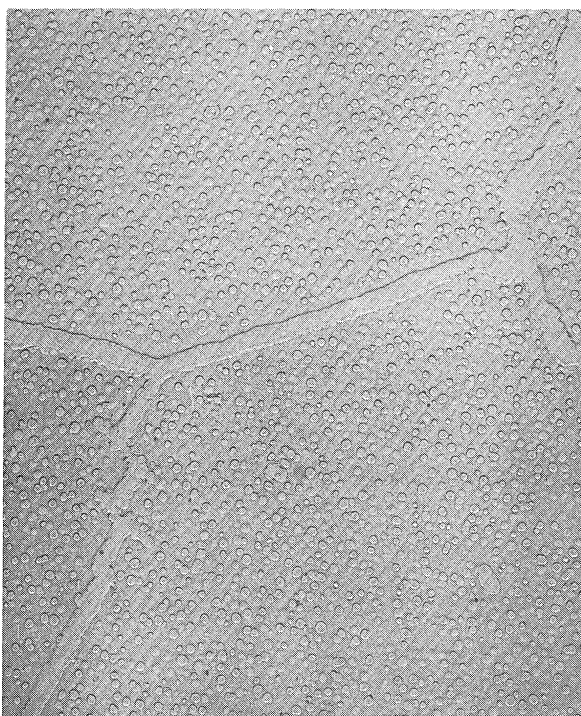
Figure 50. 5,400X Aged 10 hours at 1700°F Solution Treated 1/2-hour at 2150°F
