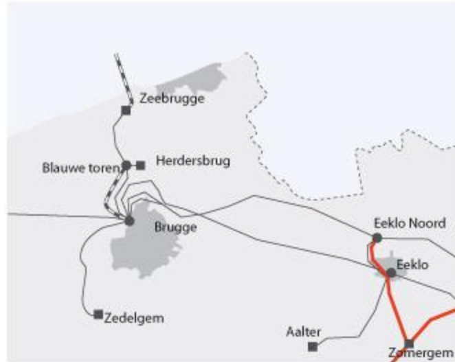
Figure 13: Belgium's Coastal Transmission Infrastructure. Belgium's transmission developer, Elia, plans to expand the 380 kV grid between the substation at Zeebrugge (upper-left) and the substation at Zomergem (lower-right). Zeebrugge is located on the Belgian coast, near an exclusive offshore wind development zone capable of hosting 2 GW of installed offshore wind power capacity. The project is expected to cost $200 million USD. 82
