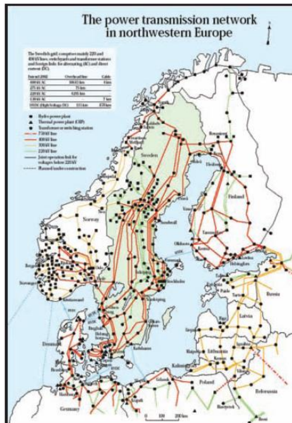
Figure 15: Sweden's Transmission Infrastructure. This transmission map details Sweden's several, large north-south transmission lines. These lines bring power from hydropower plants in the north to population centers in the south of Sweden and ultimately Poland and Germany. These north-south lines are often congested at times of peak demand. Siting offshore wind power near load centers in the south of Sweden can help to relieve that congestion by allowing more of the hydropower to flow to load centers in Poland and Germany where electricity is more costly. 91
