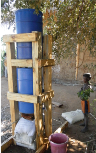
Figure 49. The basic design of our prototype water filter system with built-in storage tank. Water enters the top tank via a pump or by hand. The water then flows through ceramic candlestick filters and connection hoses into the lower storage tank. The water can then be tapped at any time with the spigot at the bottom of the storage tank. Many villagers stated they would not wait for any amount of time to clean or filter drinking water, which is the motivation behind the storage tank. Photo credit: B. Madden
