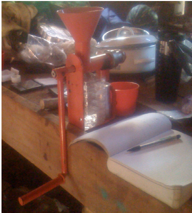
Figure 33. Seed press to determine oil yield for biofuel potential. Photo credit: B. Madden
