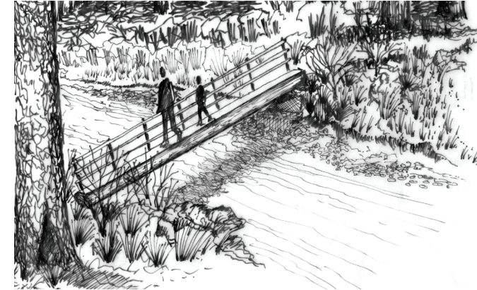
Fig. 62: Single-log stringer bridge
