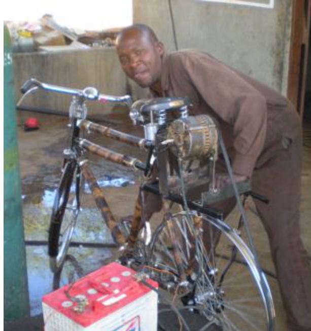
Image E-i 14: Bicycle generator being used to charge a battery at Mpala (Muhuro, 2010).
