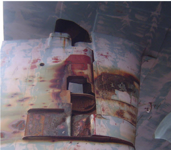
Figure 13 Cavitation erosion damage on a rudder horn (Courtesy Lloyd's Register)
