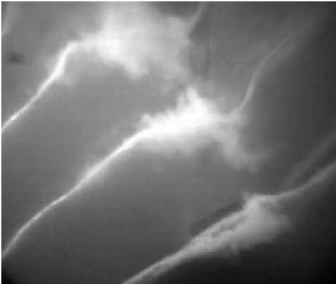
Figure 6 Breaking up tip vortex cavitation (Friesch [4])
