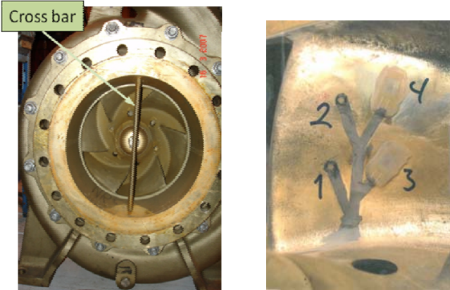
Figure 3 : Photos of pump and instrumentation of pump suction side impeller blade. Positions 1 and 2, left picture, indicate Kulite pressure transducers, 3 and 4 are strain gauges for which results are not reported in this study. The inlet diameter, upstream pipe attachment, of the pump is 350 mm.
