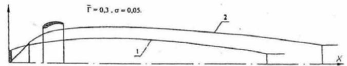
**Fig.4** Estimated cavern boundaries with positive number cavity: 1 – behind the disk, 2 – behind the cone
