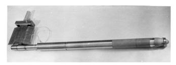
Fig.6 Model with a ring wing for towing test
