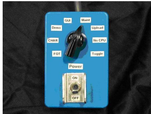
Figure 7: DAS mode control box
