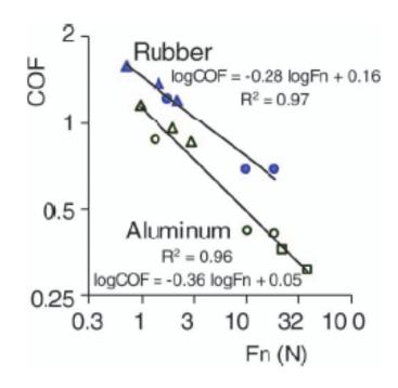
Figure 6.1.1 Friction coefficient as a function of normal force for rubber (filled symbols) and for aluminum (unfilled symbols) from three studies ( $\Delta$ ), Seo et al. accepted; (o), the present study; ( $\Box$ ), Buchholz et al. 1988) in log scales. COF = coefficient of friction. (From Seo & Armstrong, 2009)
