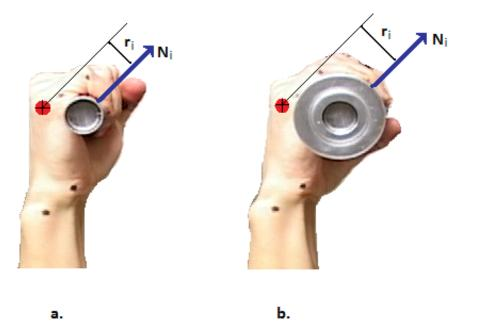
Figure 6.1.2 Normal force acting against the MCP joint for (a) 22mm and (b) 51mm handholds. The finger flexor muscles act to close the fingers creating a flexion moment about each finger joint. The surface of the handle acts against those moments. As the cylinder size increases, so does the moment arm  $(r_i)$  of a surface normal force  $(N_i)$  on the finger joint and hence increases the moment against the finger flexors. Contact area decreases as handle size decreases.
