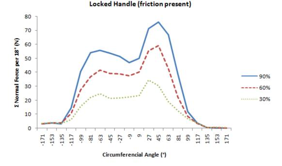
Figure 5.3.1 Integrated forces for each 18° band along long axis of handle for 30, 60 and 90% pull forces on the locked handle (friction present). The top of the handle is in the center of the graph (0°) and is the approximate location of the PIP joints. The bottom of the handle is at both ends of the graph ( $\pm$ 180°).
