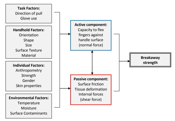
Figure 6.1.4 High-level overview of factors affecting breakaway strength. Hand/handhold coupling is comprised of both active and passive components that influence each other.
