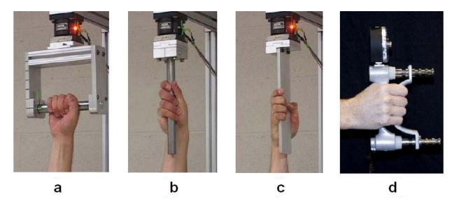
Figure 2.2.2 Handholds tested. (a) 25mm diameter horizontal cylinder (Experiment 1 and 2) (b) 25mm vertical cylinder (Experiment 1 only) (c) 64mm x 10mm vertical plate (Experiment 1 only) (d) Jamar grip dynamometer in position 2 (Experiment 1 and 2).
