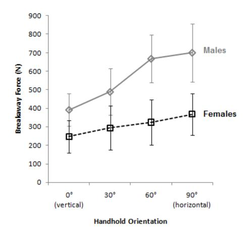
Figure 4.4.1 Mean breakaway strength (N) by orientation for male and female subjects. Strength decreases for handle orientations from horizontal to vertical.
