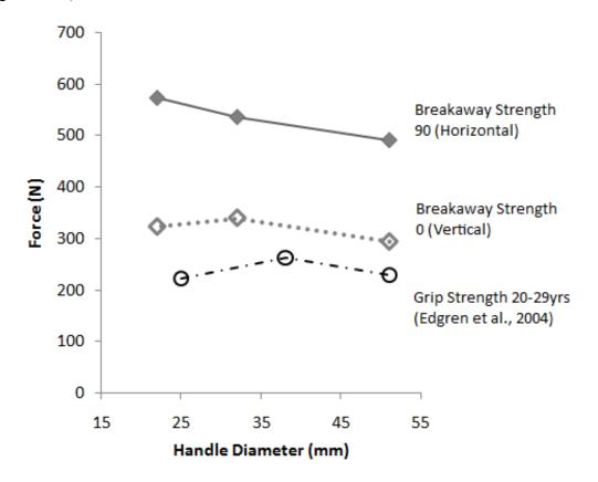
Figure 4.5.2 Mean breakaway strength vs. handhold size for horizontal and vertical handholds (Experiment 1) and voluntary isometric grip strength vs. handle size for subjects aged 20-29 from Edgren et al.. (2004). Males and females are pooled. Strength was consistently least for the largest cylinder. Strength was greatest for the 32 mm diameter handle in the vertical orientation, while strength was greatest for the smallest diameter in the horizontal orientation.
