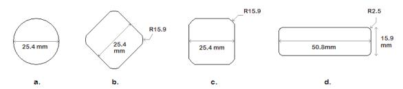
Figure 3.2.1 Handle cross-sections. (a) "cylinder": circle of diameter 25.4mm (b) "diamond": 25.4mm square rotated 45° (c) "square": 25.4mm square (d) "rectangle": 50.8x15.9 mm rectangle. R=corner radius of curvature in mm.
