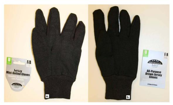
Figure 4.3.2 Gloves tested in Experiment 2 (non-dominant hand). (a) PVC dotted "high-friction" glove,  $\mu \approx 0.70$  (b) plain jersey cotton "low-friction" glove,  $\mu \approx 0.27$ . Frictional characteristics of the gloves were estimated by measuring the force at onset of movement required to pull a 1 kg aluminum plate over a gloved hand with fingers flat and palm supine.
