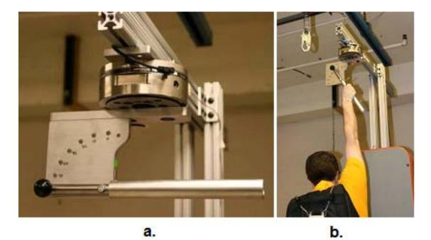
Figure 4.3.1 Experimental apparatus. a) An adjustable handle was attached to a 6-axis load cell. The handle could be adjusted to be oriented in 15° increments between horizontal and vertical. Different diameter metal cylinders can be easily interchanged. b) Subject position during breakaway trials.
