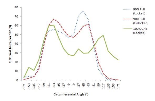
Figure 5.3.3 Integrated forces for each 18° band along long axis of handle for 90% pull forces on the locked and unlocked handles and 100% gripping effort (no pull force).
