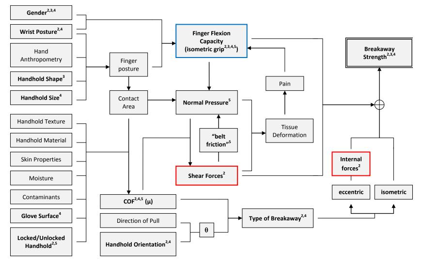
Figure 6.1.5 Schematic of factors influencing breakaway strength. Items in bold are addressed either directly or indirectly by experiments presented in this dissertation (Chapter numbers indicated by superscripts). Several factors (left side) act to generally affect either the capacity to flex the fingers (active) or the coefficient of friction (passive). Both active and passive components act to influence each other (center area) and total breakaway strength (right side).
