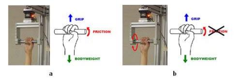
Figure 2.2.3 Breakaway handholds tested in Experiment 2. (a) Fixed 25mm horizontal cylinder. Friction resists the slipping of the hand. (b0 Unconstrained 25mm horizontal cylinder. The cylinder can rotate about the long axis, nullifying the effect of friction that would resist slipping of the hand.
