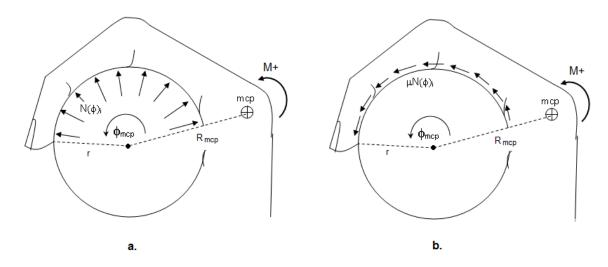
Figure 5.3.4 Illustration of parameters used to calculate resultant joint torque for the MCP joint. Normal forces (a) and frictional forces (b) over the contact arc of the finger cause a resultant moment about the MCP joint that must be balanced by internal flexion moment in order to maintain static equilibrium about the MCP joint. By definition, the joint center is at  $\varphi=0^{\circ}$ .
