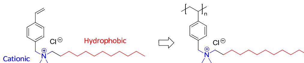
Figure I-5. Polymer disinfectants based on benzyalkonium chlorides, which are surfactants used in household cleaning products. The polymerization of this styrene derivative is a standard thermally initiated free radical process. Figure adopted from Ikeda et al (1983).
