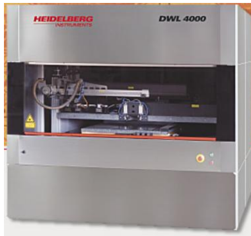
Figure 3.1 Whole view of DWL 4000 System used in this work
