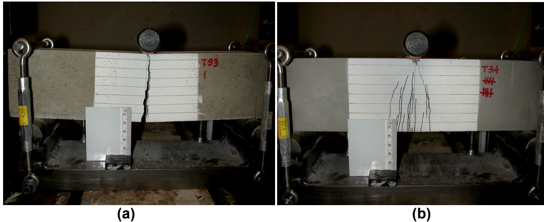
Fig. 8: Damage of (a) R/C beam after the 1 st impact (cracking penetrated through specimen) and (b) R/ECC beam after the 10 th impact (fine cracks only highlighted by a thick marker).
