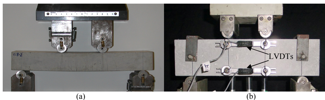
Fig. 8 Comparison of test setup for the (a) UM method and (b) JCI method (Beam deflection at the loading points was obtained from machine displacement directly in UM method).
