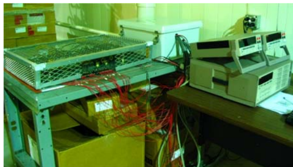
Figure 11: Fixed resistor board, junction box, source-meter, data acquisition system and switching mainframe
