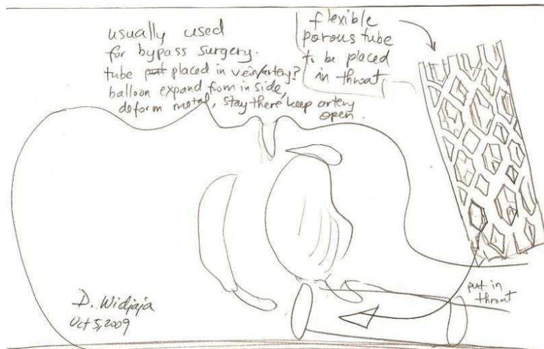
Figure 10: Physical splint design example of a semi-flexible porous tube
