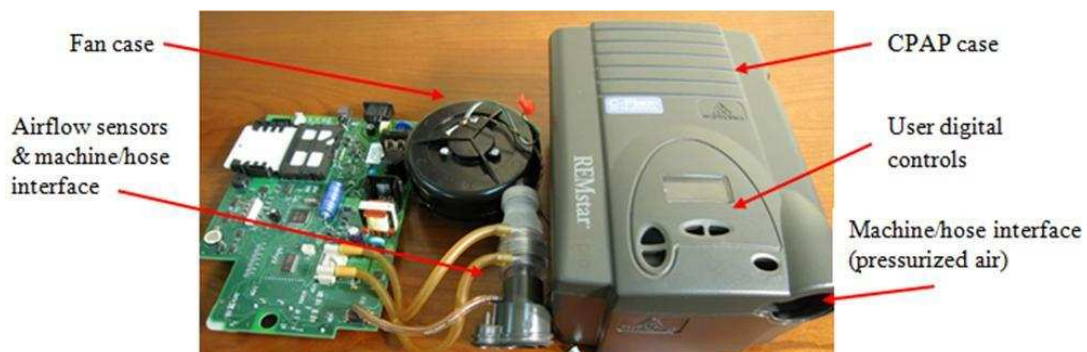
Figure 7: Disassembled CPAP machine exhibiting electrical and mechanical components
