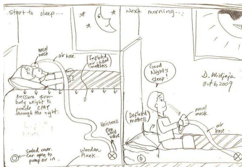
Figure 11: Constant airway pressure example design of an inflated mattress providing pressure
