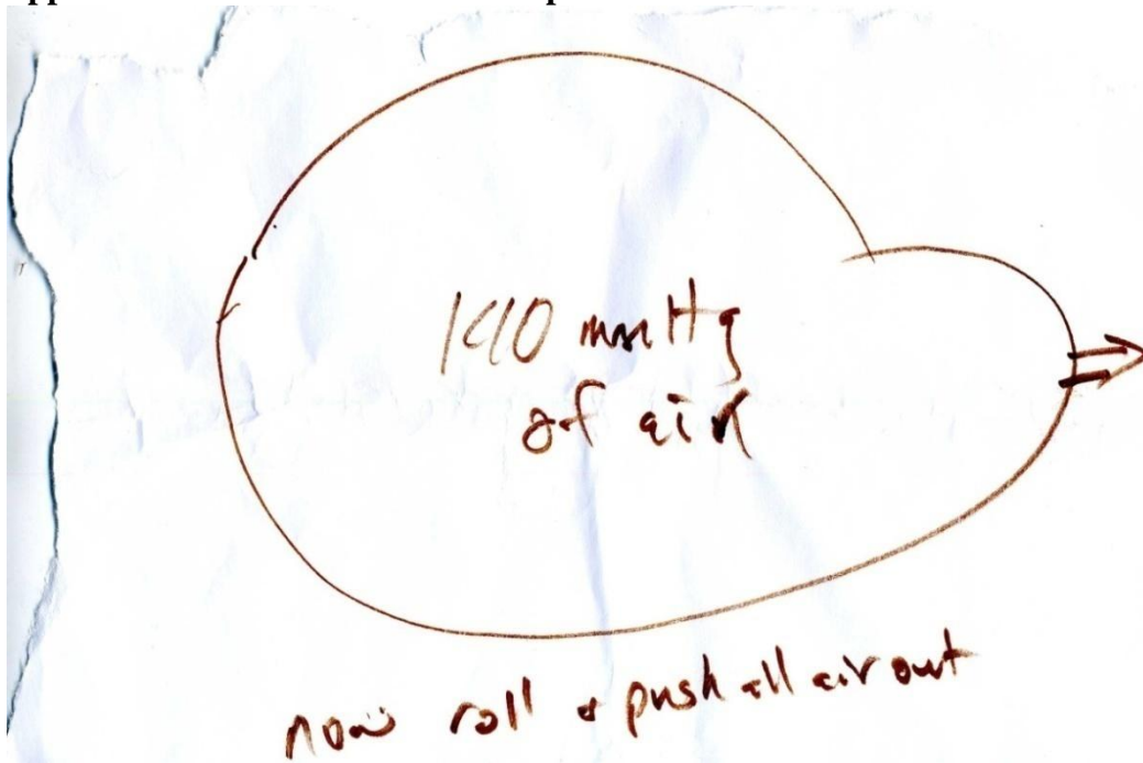
Figure 1: Balloon- The intention of this idea is to use a balloon that has 140 mmHg of air initially, and is attached to the cuff. The balloon is squeezed and the cuff is inflated to 140 mmHg.
