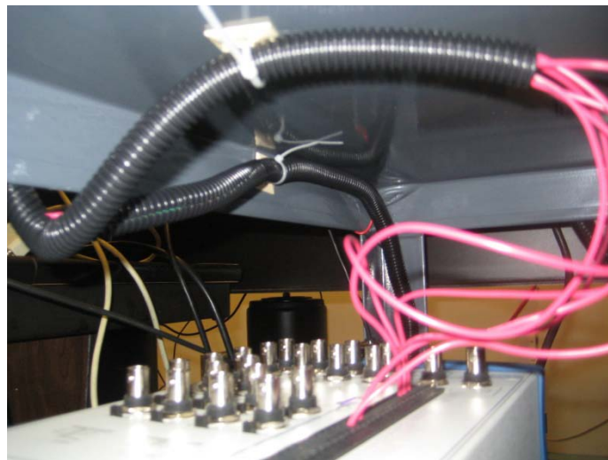
Figure 4: Wrapped and Zip Tied DAQ Connections
