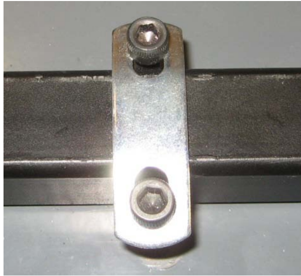
Figure 19: Fixtures keeping mechanism on the cart
