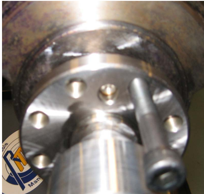
Figure 8: Location of pin installation
