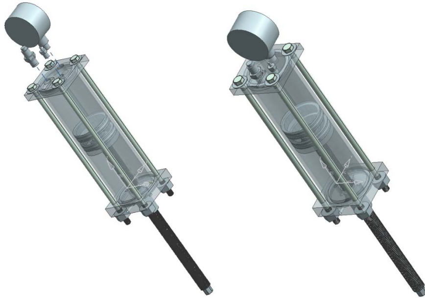
Figure 11.4: Final assembly, exploded view (left), assembled (right)
