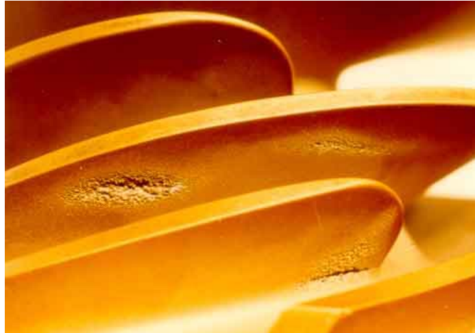
Figure 4.1: Damage on a mixed flow pump blade caused by cavitation [6]
