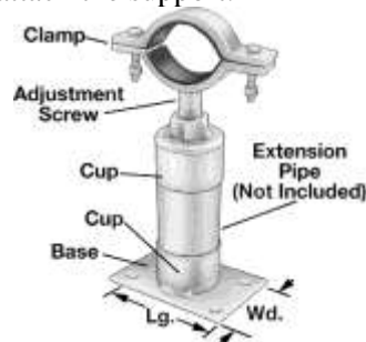
Figure 31. Schematic of Clamp Style piping support (28)
