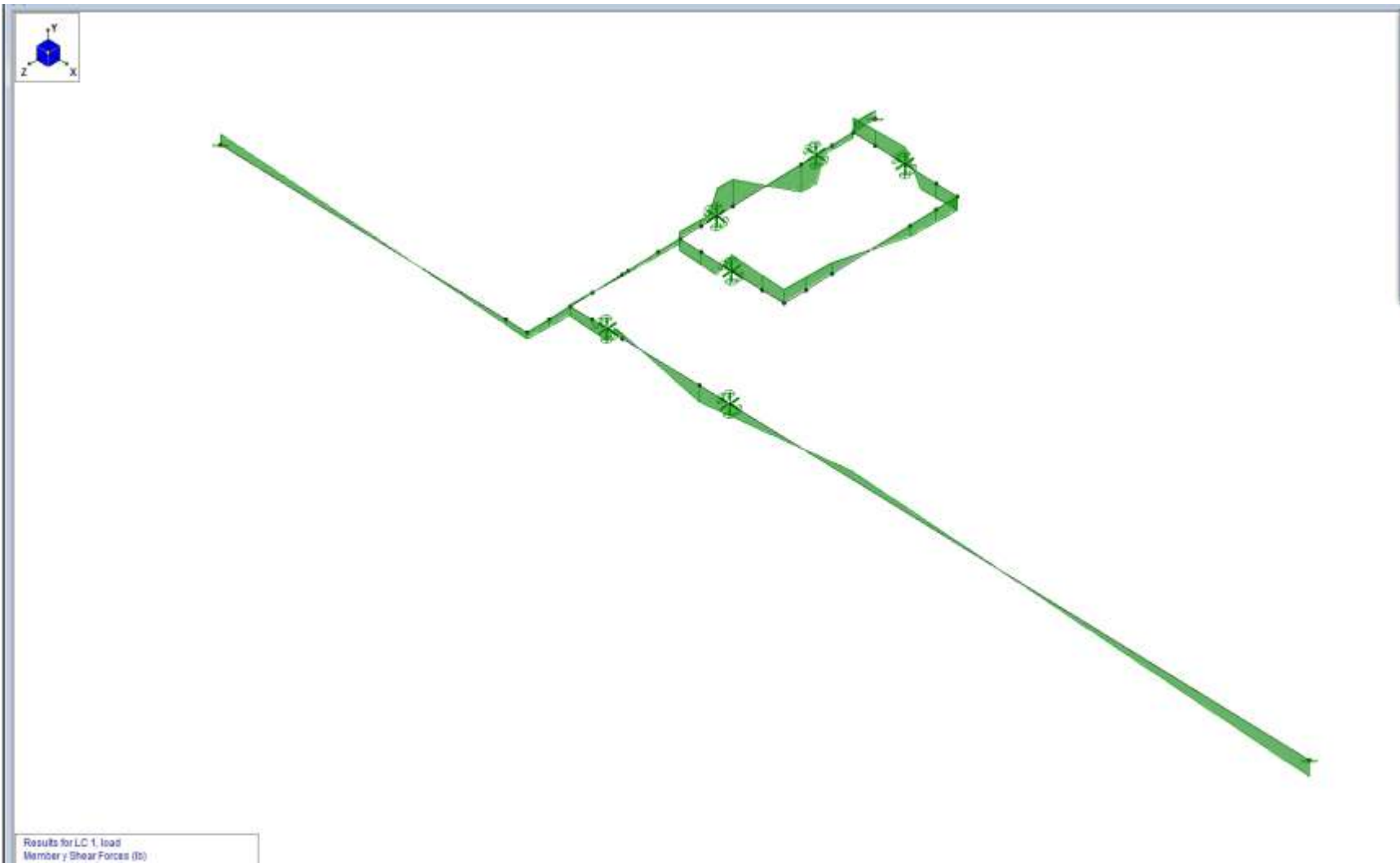
Figure 100: y Shear force distribution in the stand pipe sector
