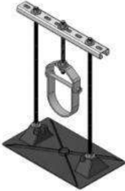
Figure 33. Schematic of Pipe Hangers piping support (28)
