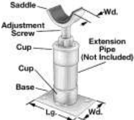
Figure 32. Schematic of Saddle Style piping support (27)
