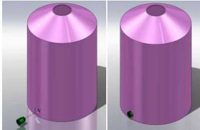
Figure 88 PVC coupling to Stand Pipe Assembly
