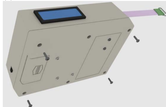
(b) Four screws in four corners of bottom of case
