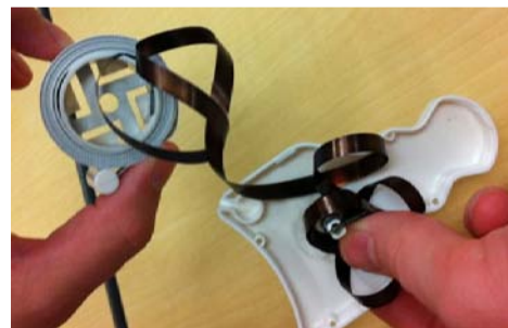
Figure 12: Thin, metallic tape which generates the constant tension in the Myotape
