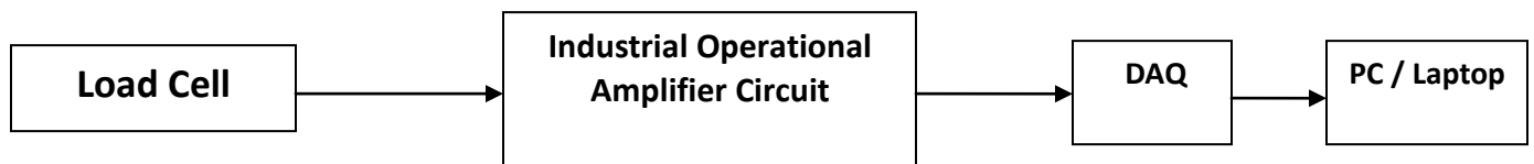
Figure 40: Load cell amplifier circuit
