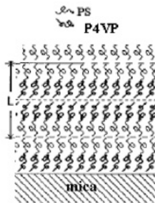
Figure 6.4 Illustration of the bulk lamellar length for a PS-PVP ( f_{PS} = 0.51 ) film on mica. Image reproduced from Zhao. 4
