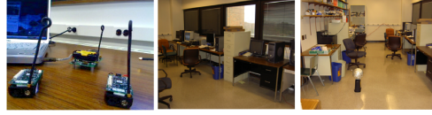
Figure 3.4: Experimental platform: wireless Mica2 sensor nodes.
