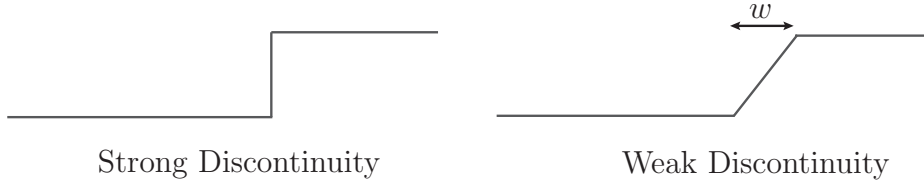
Figure 4.1: Schematic of displacement field in a domain containing strong and weak discontinuities. w is the width of the diffused band.
