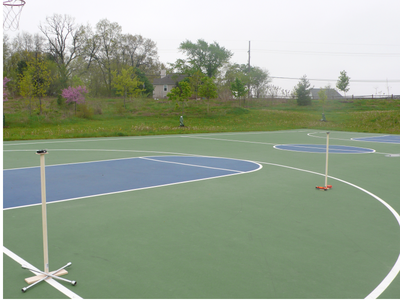
Figure 6.9: Basketball court where we validate the Two-Ray signal propagation model.
