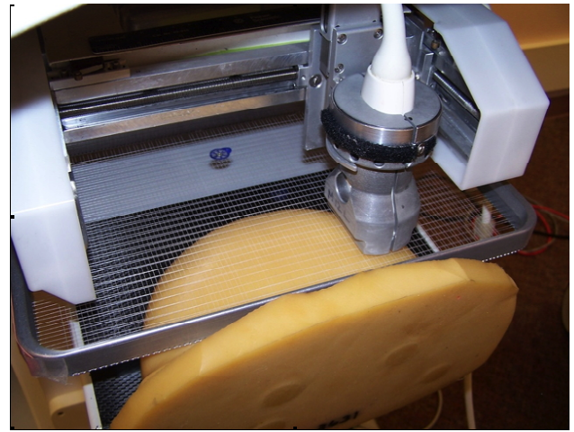
Figure 1. Existing Ultrasound system for scanning a breast phantom, stabilized by a fiber mesh and its frame over the x-ray detector (black). After x-ray TM, the US scanning frame is rotated into place over the breast. Coupling gel is not yet applied. The transducer's vertical position can be fixed, spring loaded, or manually controlled for local compression.
